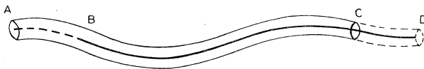
FIG. 1. The chain moves to the right, and a certain portion ( A, B ) of the original tube disappears; a new part of the tube ( C, D ) is created.
